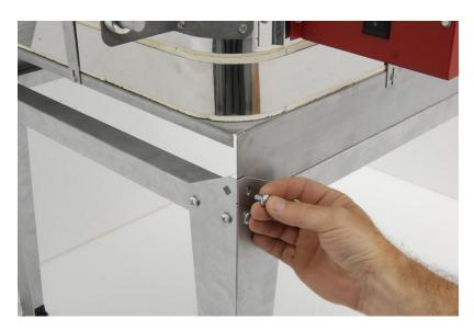
Insert a bolt through each front leg and kiln base and secure with nut.
