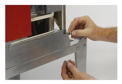
Insert a bolt through each side of rear base and stand frame angle and secure with nut.
