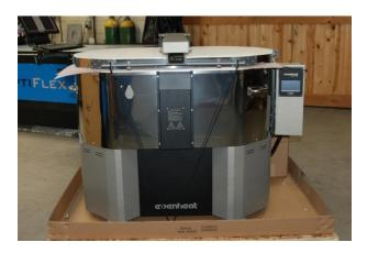
Your Evenheat GTS unit sits on top of a metal base, the base is shipped attached to the kiln. This structure is designed to support the weight of the kiln as well as any work inside. The base provides sturdy support for you kiln.
