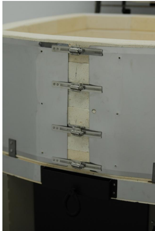
Figure 4 - Expose Jacket Clamps
