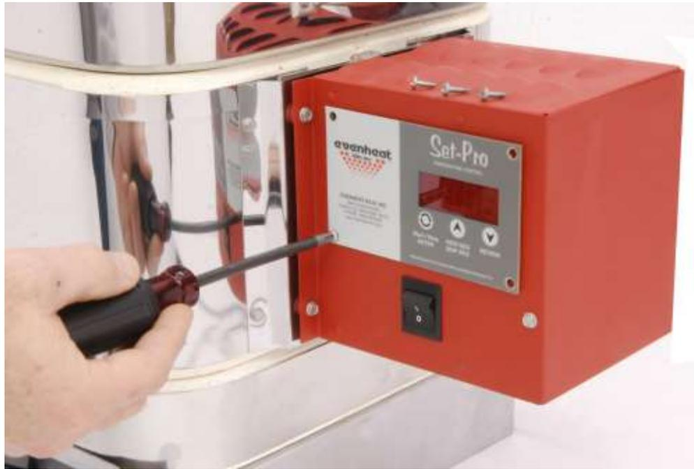
Remove the 4 screws that secure the kiln controller to the control enclosure as shown.
