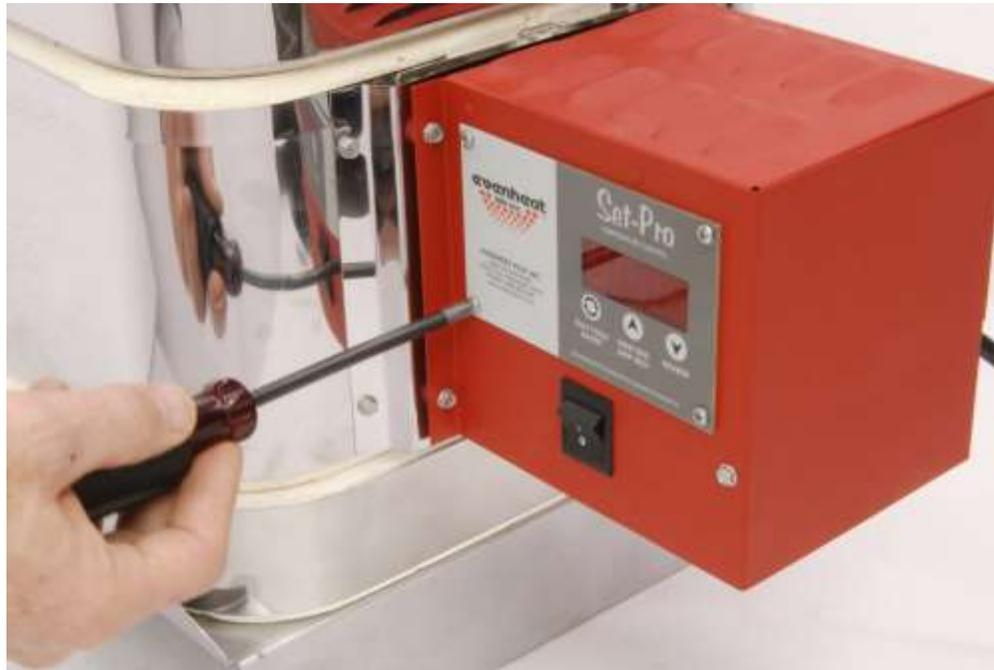
Place the control back into the control enclosure and secure with screws as shown.
