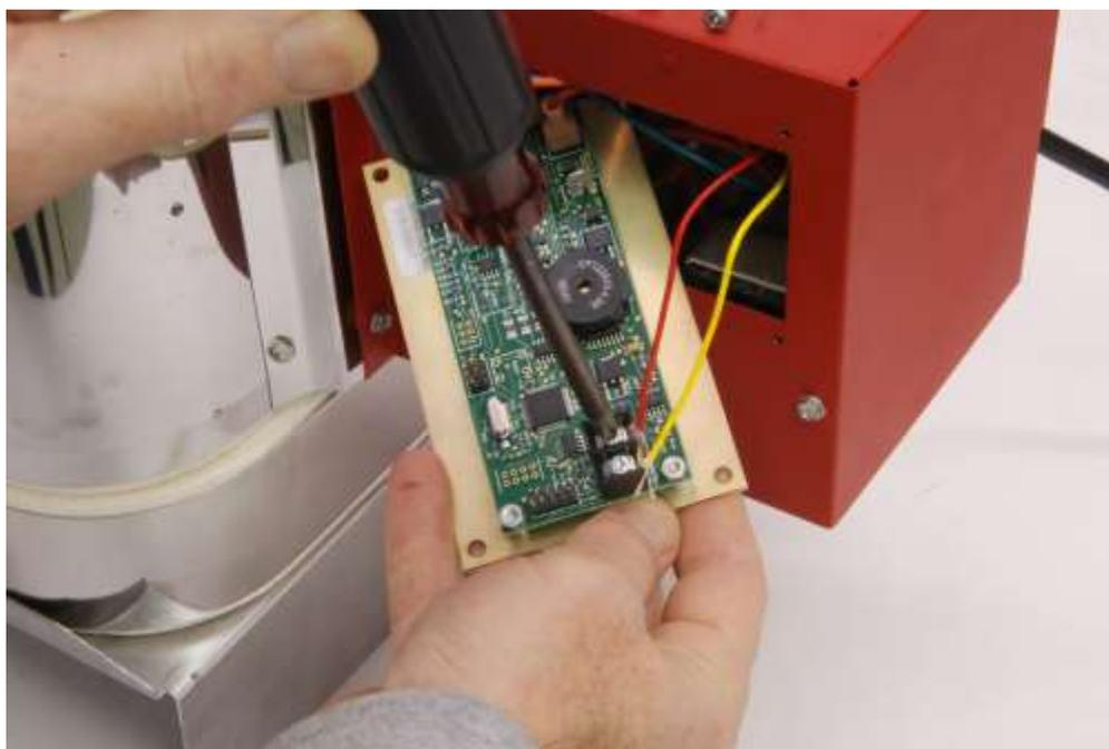
Connect the new thermocouple wires to the controller as shown. *Be mindful to connect the Red colored wire to the Red colored connection point (which is marked). Obviously the Yellow wire goes to the other connection point. If you hook it up backwards improper reading will result and you don't want to do that.*
