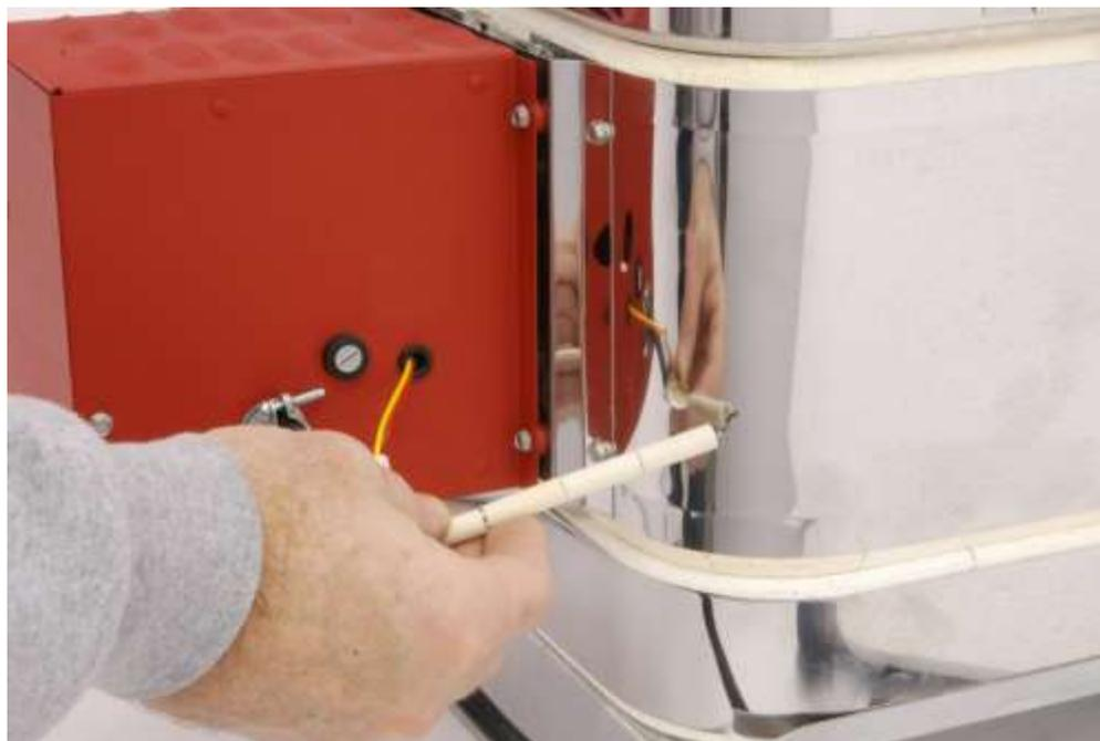
Pull the old thermocouple from the kiln as shown.
